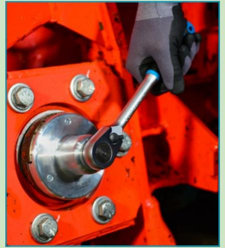
Operating using ratchet with inserted 1/2" (12.5 mm) 4-point socket
