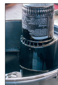
With drainer for oil filter
