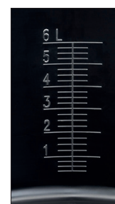
Internal scale in litres and US gal/ UK gal
