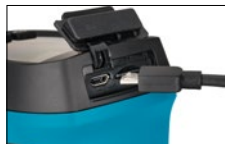
Power supply: USB cable (Micro USB)
